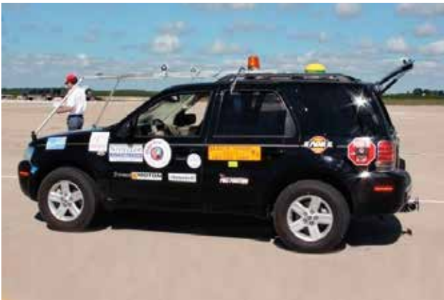
FIGURE 2. A DARPA Urban Challenge vehicle, utilizing a low-cost vision system comprising mainly of personal computer webcams.
